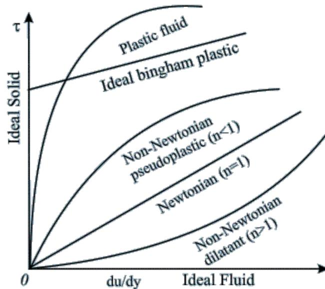
Figure 3: Shear stress and deformation rate relationship (NPTEL)
